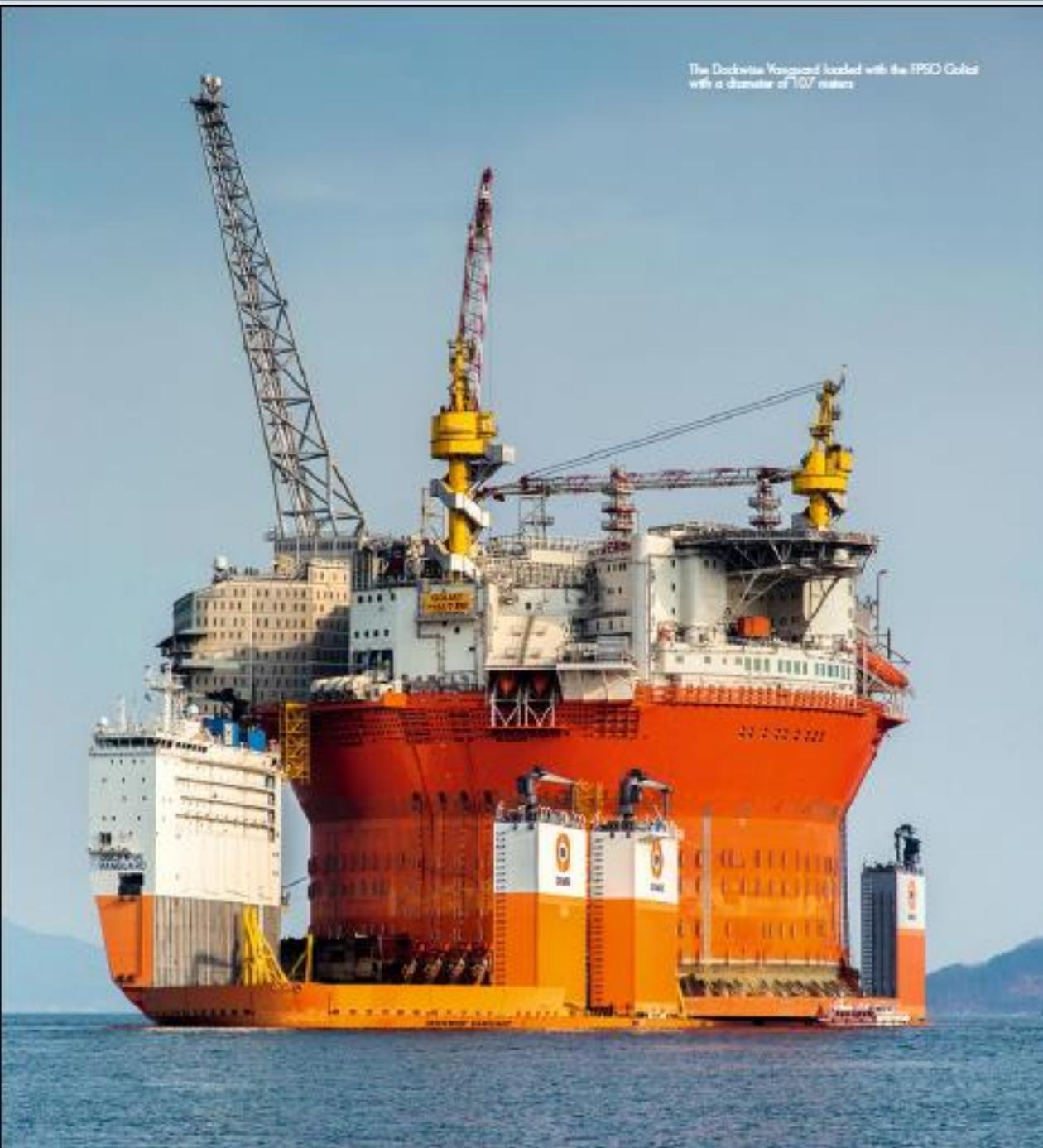
The Dockwise Vanguard loaded with the FPSO Galica with a diameter of 107 meters
